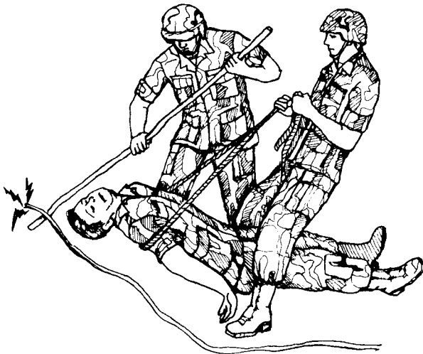
Figure 3-34. Casualty removed from electrical source (using nonconductive material).
