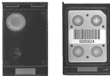
Figure 1: DT-648 Open holder with TLD card inside
