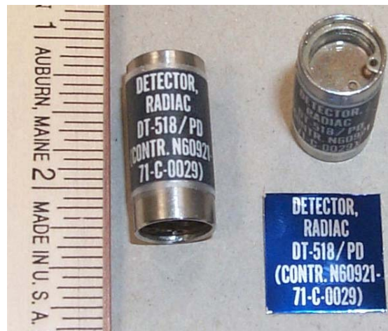
Figure 7. Photograph of the DT-518/ PD accident dosimeter. The scale shown is in inches.
